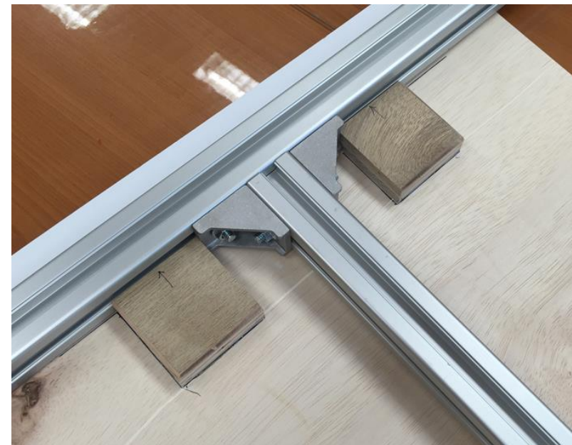
Runway stabilization guide in place
